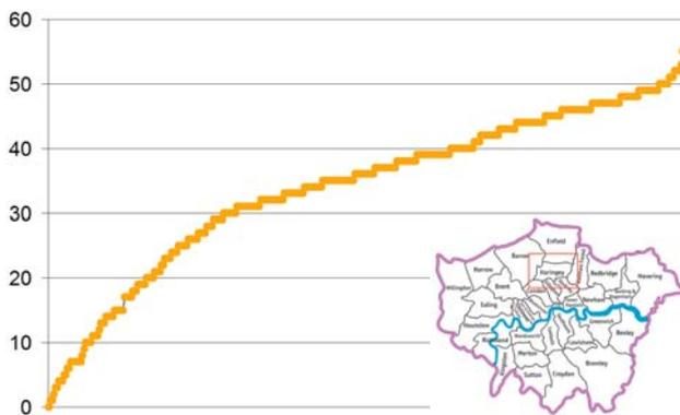
Distribution of soils in terms of their Plasticity Index. The maximum PI is 55% and the average PI is 34%. See bar graph below for breakdown.
